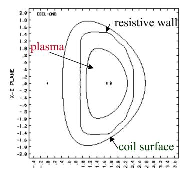
**VACUUM** model includes plasma, wall, and coil surface
