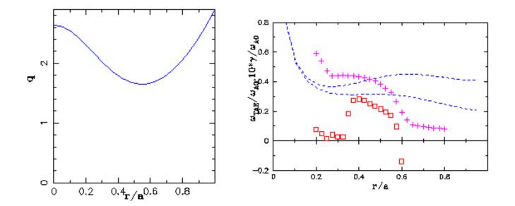
RTAE is found near  $q_{min}$  at critical  $\beta_{0\alpha\sigma rit} = 0.23\%$  at r/a = 0.4, (local  $\beta_{\alpha} = 0.047\%$ ). NO relaxed RTAE stable profiles were found. Alphas will be trasported outside  $q_{min}$  surface.
