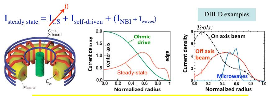
Off-axis current sources are Lower Hybrid Current Drive (LHCD, neutral beams (NBCD) & microwave driven currents (ECCD)
