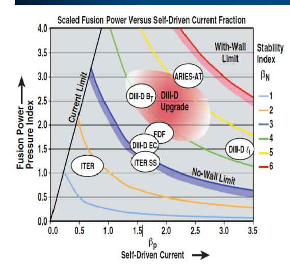
• Simultaneous achievement of high pressure and high self driven current requires high stability index
