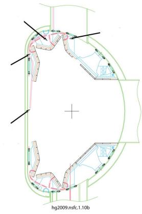
DOME D<sub>2</sub> puffing has highest fuelling efficiency, less from inner target plate, lowest from outer target plate. Compared to SN configuration, DN is more sensitive to gas puffing location.
