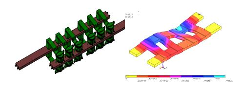
**Converter arm displacement in EM force**
