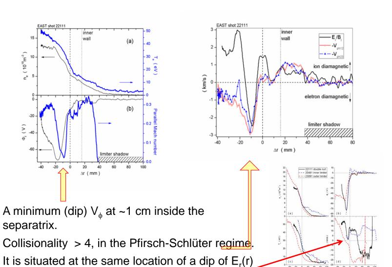
• But a dip of  $V_{\phi}(r)$  not observed in the discharges that the plasma edge touches the outer limiter
