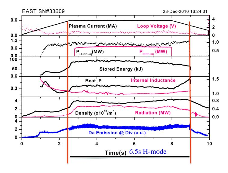
H-mode during ramp-up, flat-top and ramp-down phases, very important for ITER
