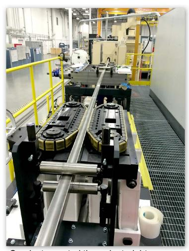
Conductor routed through straightener
