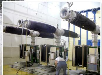
One of four sets of 400kV, 3-phase HV circuit breakers undergoing factory acceptance test at Alstom SAS, Villeurbane, France
