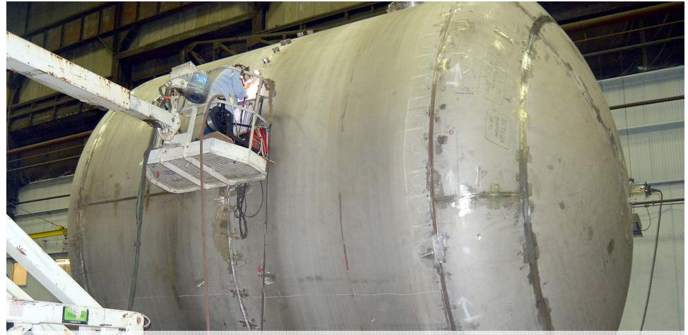
First of four 61,000 gallon drain tanks nears completion at Joseph Oat in Camden, New Jersey. (Fifth tank Is ~30,000 gallons) Photo: US ITER
