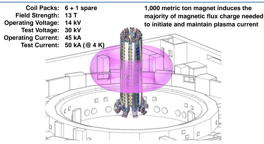
The most powerful pulsed superconducting electromagnet in history (5.5 Gigajoule stored energy capacity)
