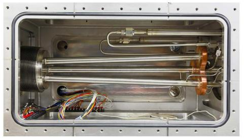
3-barrel unit prototype for disruption mitigation
