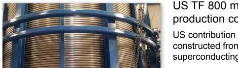
US TF 800 m Dummy Conductor and 100 m production conductor delivered to EU winding facility
