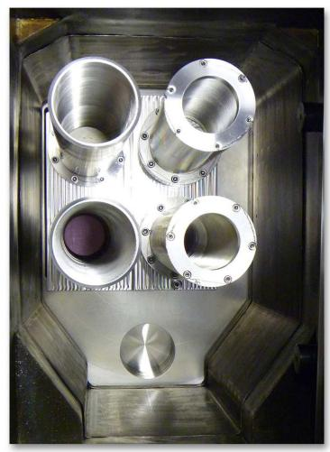
Prototype antenna for the low-field side reflectometer installed on DIII-D.
