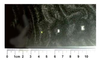
Small pellets fro ELM pacing and larger pellets for D/T fueling
