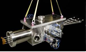
Pellet guide tube selector test unit
