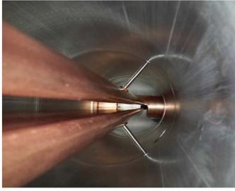
Four-port 50/50 Power splitter on the test bench. Internal view of outer conductor (AI) and inner conductors (CU) of the power splitter (Mega Industries, Portland, Maine)
