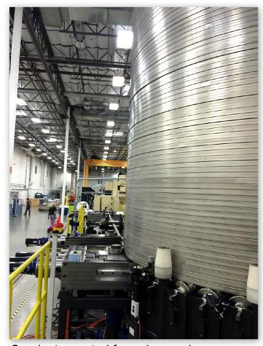
Conductor routed from de-spooler
