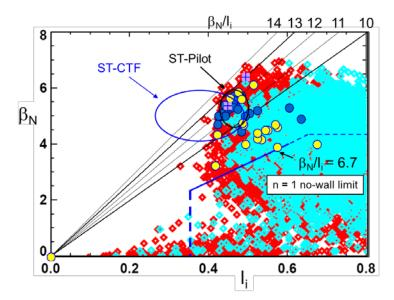
Figure 2: Operational stability space  $(l_i,\beta_N)$  in NSTX illustrating a higher number of disruptions (yellow circles) at intermediate values of  $\beta_N$  in dedicated control experiments. The sharp reduction of the n = 1 ideal no-wall stability limit as  $l_i$  is decreased is also shown, the vertical dashed line representing the approximate computed current-driven kink limit.
