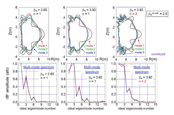
Figure 3: Multi-mode RWM analysis of ITER advanced scenario discharges, demonstrating a significant eigenmode spectrum in addition to the standard single ideal eigenmode typically assumed in control calculations.
