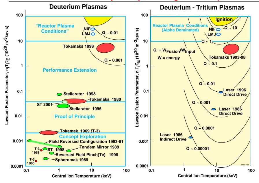
Only the tokamak is sufficiently advanced to permit the design, construction and initiation of a next step burning plasma experiment within the next decade that could address the alpha-dominated burning-plasma physics issues of magnetic fusion.
