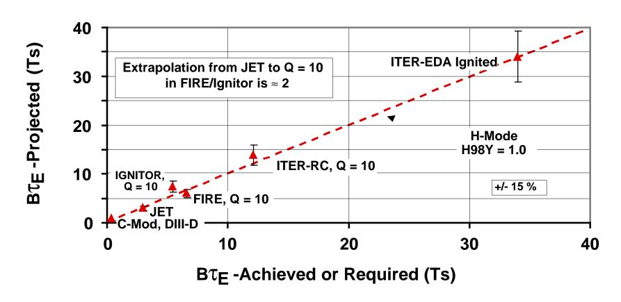
High magnetic field allows FIRE and IGNITOR to operate at high density, thereby reducing the required extrapolation in confinement, the most uncertain quantity.
