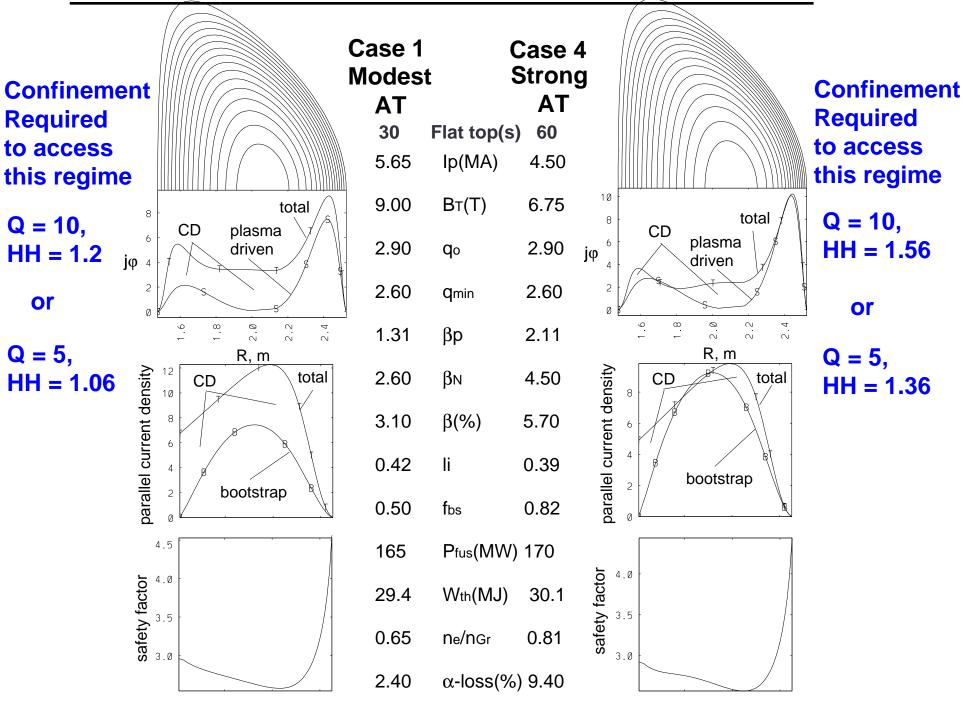
The transport calculations assumed 150 MW of fusion power and n(0)/< n > = 1.5.
