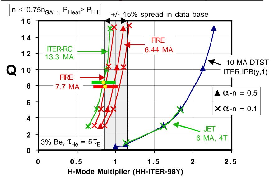
The baseline FIRE(6.44 MA) can access the alpha-dominated regime (Q > 5). FIRE could be extended to 7.7 MA to provide increased margin equal to ITER-RC.
