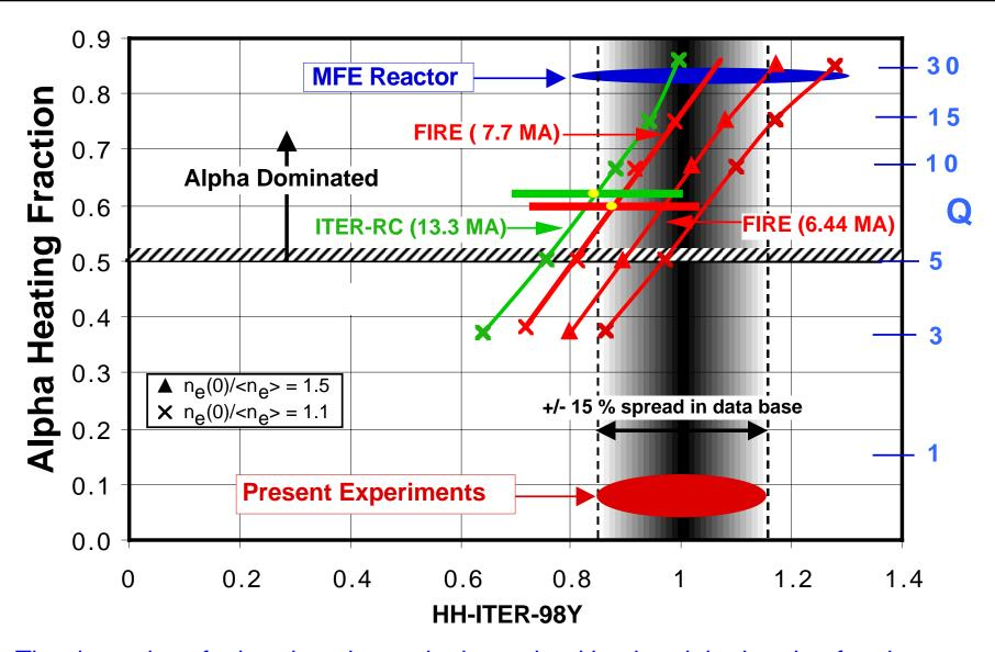
The dynamics of a burning plasma is determined by the alpha heating fraction which is not subject to a sharp threshold versus confinement.
