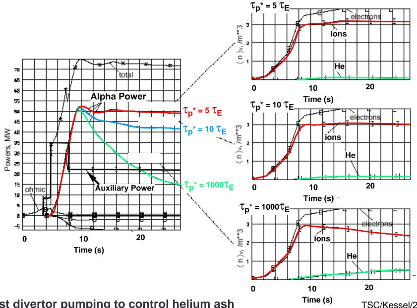
Adjust divertor pumping to control helium ash
