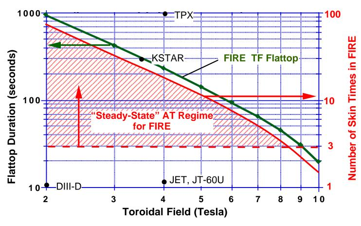
Note: FIRE is  $\approx$  the same size as TPX and KSTAR. At Q = 10 parameters, typical skin time in FIRE is 13 s and is 200 s in ITER-RC.
