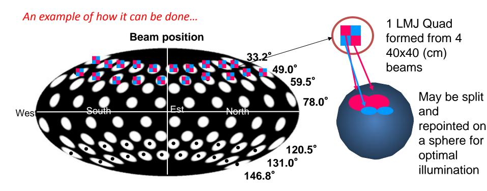
40 quads pattern: - uses quad splitting, defocusing and repointing (Polar Drive)
