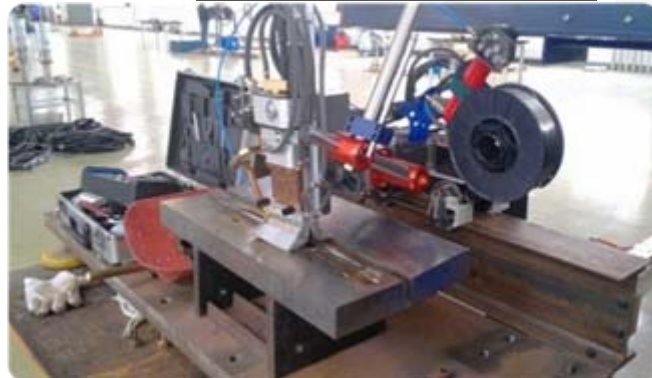
R&D of Narrow Gap TIG Welding on VV 窄间隙焊接预研 试验
