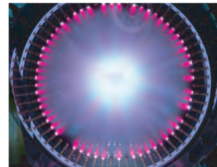
Plasma-jet liner (Witherspoon et al.)
