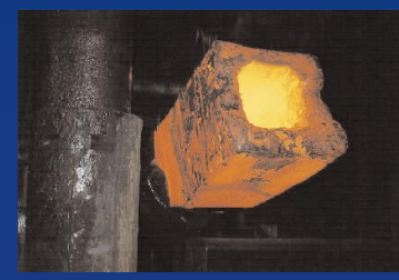
Inner leg case section during forging as a hollow tube, before cutting into two U sections (Kind).
