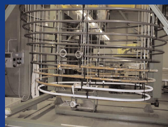
Conductor after heat treatment, opened out by ‘unspringing’ to give space to wrap with insulation without damaging the superconductor. The insulation has been applied to the lower turns (Ansaldo Energia).
