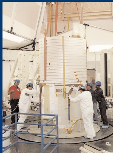
Transfer of a layer onto a coil assembly to form the inner module at Lockheed Martin.
