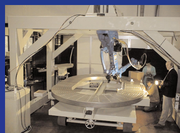
The top of the groove is closed by a cover plate which is laser welded into position (RTM).
