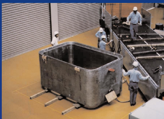
Equatorial port extension shipped from the RF to the test site at JAERI Naka for integration testing.
