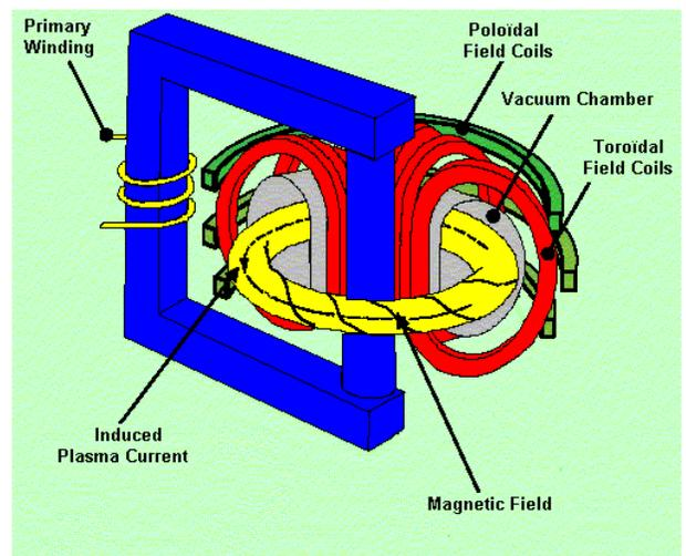
Figure 1 : Tokamak configuration
