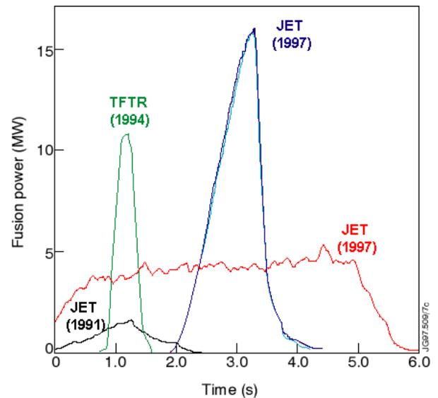
Figure 3 : JET and TFTR performance on D-T operation
