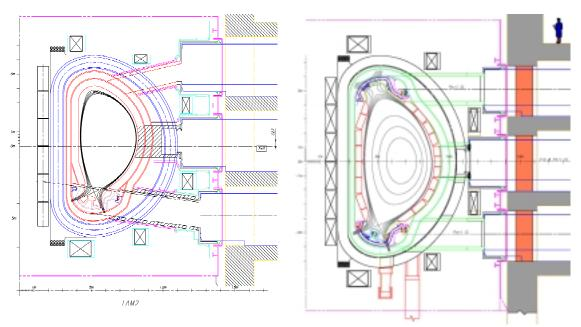
Fig 1a. Cross section of IAM design.
