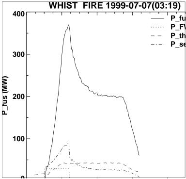
Fig. 2.5.1. FIRE example of start-up, burn and termination.
