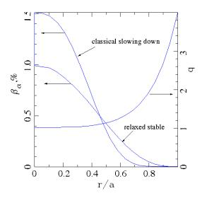
Fig. 2.1.1. Alpha particle slowing down beta profile vs. minor radius for a circular equilibrium with parameters typical of a compact high field plasma: B=10T, R=2.5m, a=0.5m,  $ne(0)=5x10^{14}cm-3$ , T(0)=20keV, and a 50-50 d-t mixture. The  $\beta\alpha$  profile is predicted to be unstable according to the HINST code. However, the relaxed profile is stable. (Figure courtesy of N.N. Gorelenkov).
