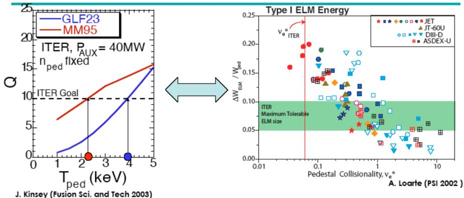
Burning plasma performance dependence on pedestal pressure varies with stiffness of the core transport model  Low collisionality pedestals in current devices usually result in large ELMs that are incompatible with a burning plasma first wall
