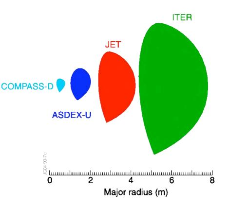
Cross sections of present EU D-shape tokamaks compared to the cross section of ITER
