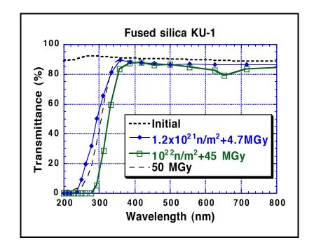
Measured transparency of KU1 fused silica (8 mm thick): as a function of wavelength for different neutron and gamma fluxes after irradiation in a nuclear reactor at  $T = 180^{\circ}C$  and with a  $Co^{60}$  gamma source at a room temperature [D.V.Orlinski. in J. Problems of Atomic Science and Engineering (in Russian), series – Nuclear fusion, v.2, 2000, p.21 – 39].
