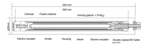
Schematic diagram of typical microfission chamber. Fissile material, such as  $^{235}$ U, is coated on the cylindrical electrode. The ionizing gas between the electrodes is Ar + 5% N<sub>2</sub> (14.6 atm) [T Nishitani et al, Rev Sci Instrum 70 No 1 (1999) 1141]
