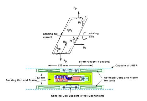
Principle of Operation and Prototype Implementation of the Load Cell Type Steady State Magnetic Sensor [S Hara, et al., Rev Sci Instrum 70 No 1 (1999) 435.].
