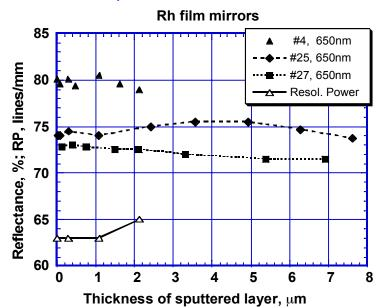
Dependences on sputtered layer thickness of reflectance at  $\lambda$  = 650 nm and resolving power versus thickness of sputtered layer for Rh film on copper substrate mirrors. [V S Voitsenya et al, Rev. Sci. Instrum, vol. 72 No 1, 475, (2001)]
