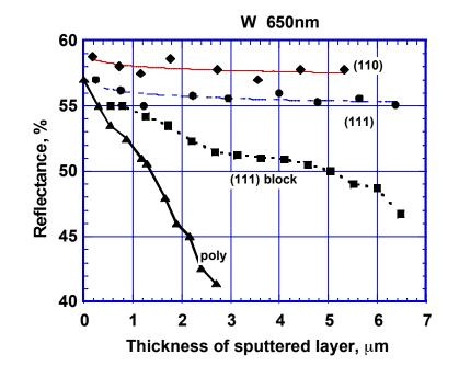
Reflectance of W mirrors (polycrystal, block monocrystal and real monocrystals with two planes of orientation) at  $\lambda$  = 650 nm depending on the sputtered layer thickness. [V S Voitsenya et al, Rev. Sci. Instrum, vol. 72 No 1, 475, (2001)]
