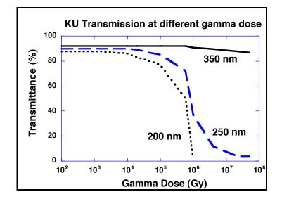
Measured transparency of KU1 fused silica (8 mm thick): as a function of gamma dose at three wavelengths after irradiation with a  $Co^{60}$  gamma source at a room temperature [D.V.Orlinski. in J. Problems of Atomic Science and Engineering (in Russian), series – Nuclear fusion, v.2, 2000, p.21 – 39].
