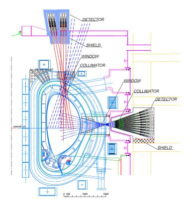
Schematic of Radial and Vertical Neutron Cameras. The Sight-lines for the Vertical Camera will be distributed at Four Different Toroidal Locations [K Ebisawa et al, Rev. Sci. Instrum, vol. 72 No 1, 545, (2001)].
