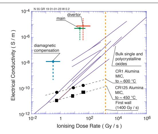
Measured Radiation-Induced Conductivity in bulk single and polycrystalline oxides, and MI Cables as a function of Ionising Dose Rate combined with magnetic diagnostic requirements at selected locations. The vertical bars represent the range of design values of RIC that can be tolerated for each coil; the horizontal bars represent the uncertainty on the flux.
