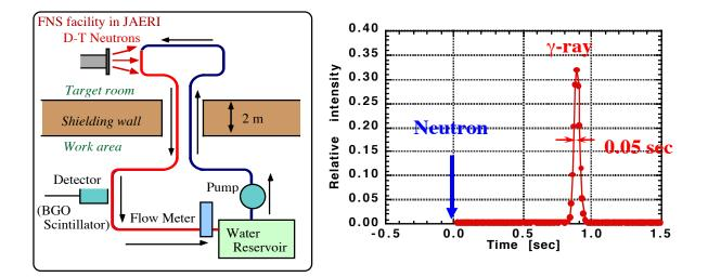
Schematic of the experimental test of the Fluid Flow Activation technique and some initial results [Y. Uno, et al., to be published in Fusion Eng. Design]
