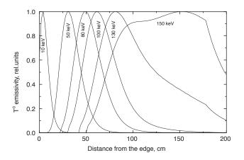
Calculated emissivity functions for T and typical ITER-FEAT conditions showing that with the upgraded NPA detector measurements of  $n_T/n_D$  should be possible into the central region [A.I.Kislyakov et al, in 'Diagnostics for Experimental Thermonuclear Fusion Reactors 2', ed. P.E. Stott, G. Gorini, and E. Sindoni, Plenum Press, New York, p.353 (1998).
