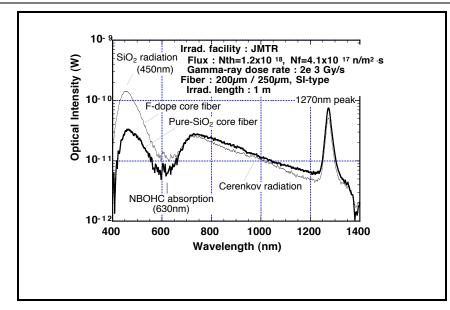
Cerenkov radiation from optical fibre under fission neutron irradiation.
