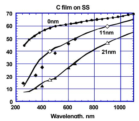
Experimentally measured (solid points) and calculated (lines with corresponding open markers) spectral dependencies of effective reflectance for clean SS and for SS with carbon coating of thickness indicated near every curve. [V S Voitsenya et al, Rev. Sci. Instrum, vol. 72 No 1, 475, (2001)].
