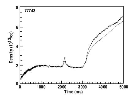
The electron density measured with a conventional interferometer (noisier curve) and the ion mass density measured from the Alfvén speed curve (quieter curve) on DIIID [H. Ikezi, et al, Rev. Sci. Instrum. 68, 478 (1997)].
