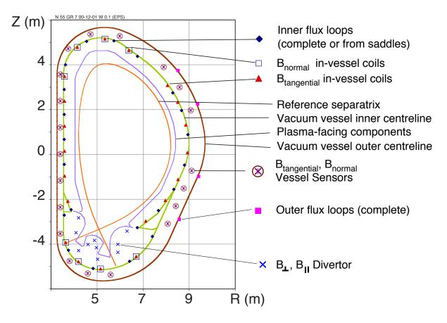
Poloidal Distribution of Magnetic Sensors. The diamagnetic loops and external Rogowski coils are not shown. [K Ebisawa et al, Rev. Sci. Instrum, vol. 72 No 1, 545, (2001)].
