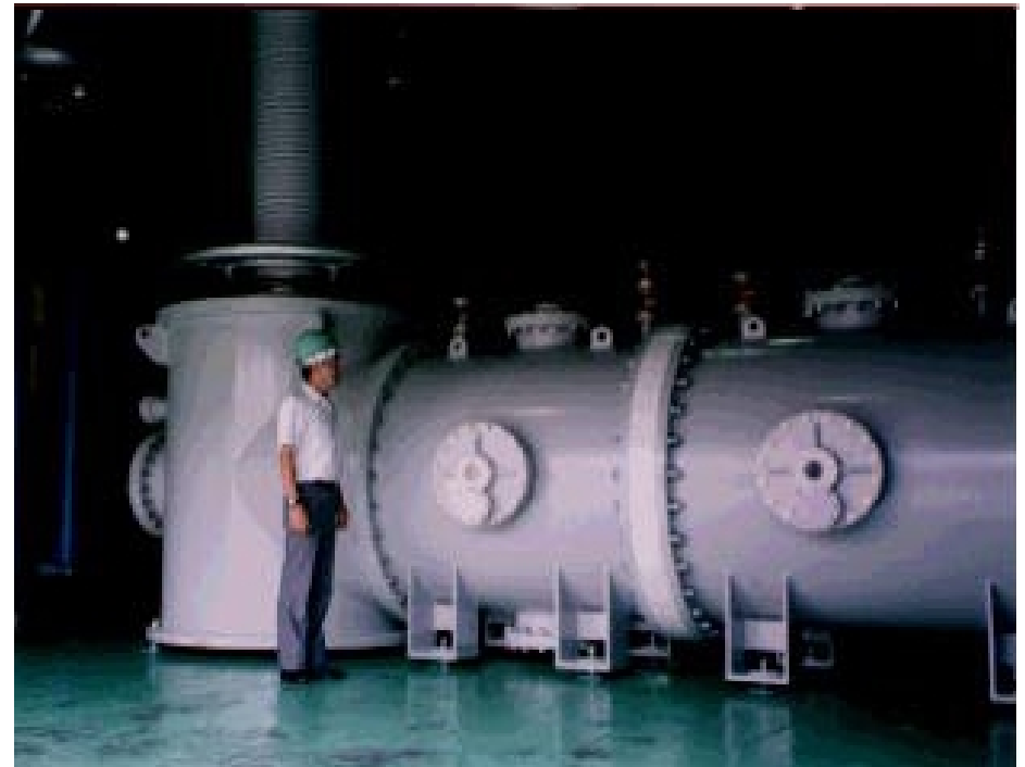
Test facility for the mockup bushing, located between two SF 6 tanks
