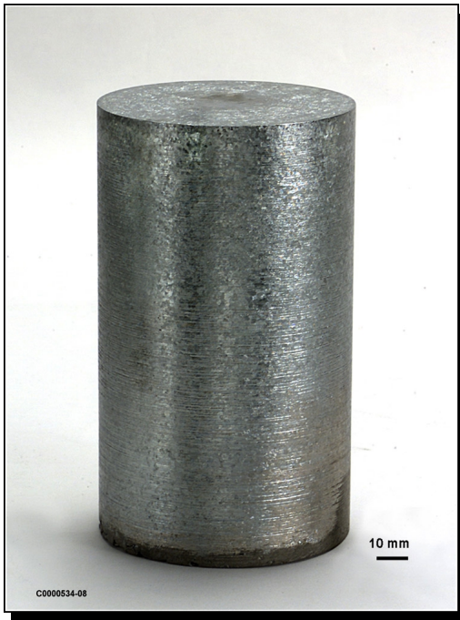
Ingots of arc melted Mo-Re are routinely processed from powder
