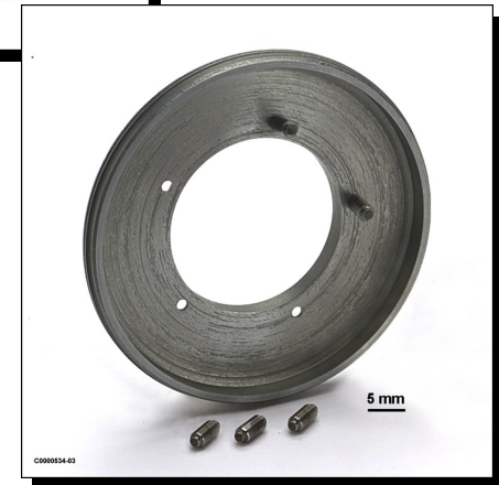
These ingots have been fabricated into precision components by extrusion, rolling, and machining
