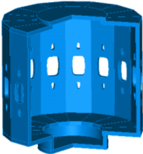
Polyurethane foam insulation with fiberglass inner and outer skins
