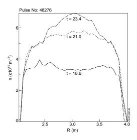
Fig. 3. The electron density profile at three times.
