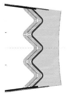
Concerning the toroïdal field coils, the use of mineral insulators would authorize the decrease of the thickness of the shielding, on the high field side, to a value of 0.2 to 0.3 m. In view of the high level of irradiation, no impregnation under vacuum with resins would be envisaged. Moreover, the coils would not be cooled by water but by organic fluids.
