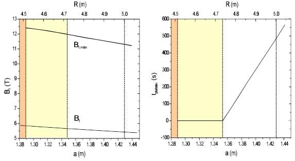
Figure 3.1.1: Magnetic field in the plasma, in the superconductor and duration of current plateau corresponding to machines of increasing dimensions, for A=3.5, obtained by the optimization algorithm.
