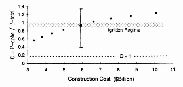
Fig. IV.1. Performance vs. cost for super-conducting ITER designs.
