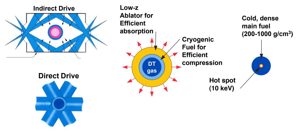
Inertial Confinement Fusion uses direct or indirect drive to couple driver energy to the fuel capsule Spherical ablation with pulse shaping results in a rocket-like implosion of near Fermi-degenerate fuel
