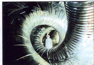
Inside story. Iiyoshi with a model of the Large Helical Device, in which helical coils create a powerful magnetic field to confine burning plasma.
