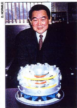
Inside story. Iiyoshi with a model of the Large Helical Device, in which helical coils create a powerful magnetic field to confine burning plasma.
