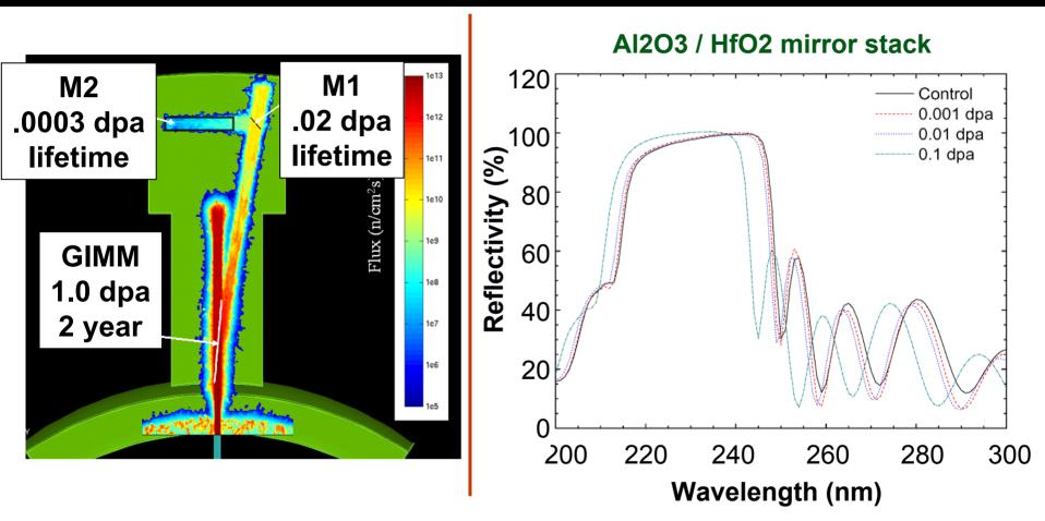
The "key" Match irradiation-induced dimensional changes in substrate and mirror layers
