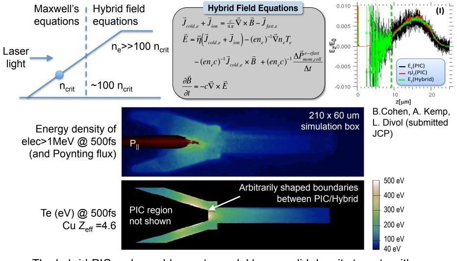
The hybrid-PIC code enables us to model large, solid density targets with a realistic self-consistent electron distribution
