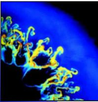
3D kinetic PIC code PSC (solves full Maxwell's equations for fields and kinetic particles, with v. high spatial, temporal resolution)
