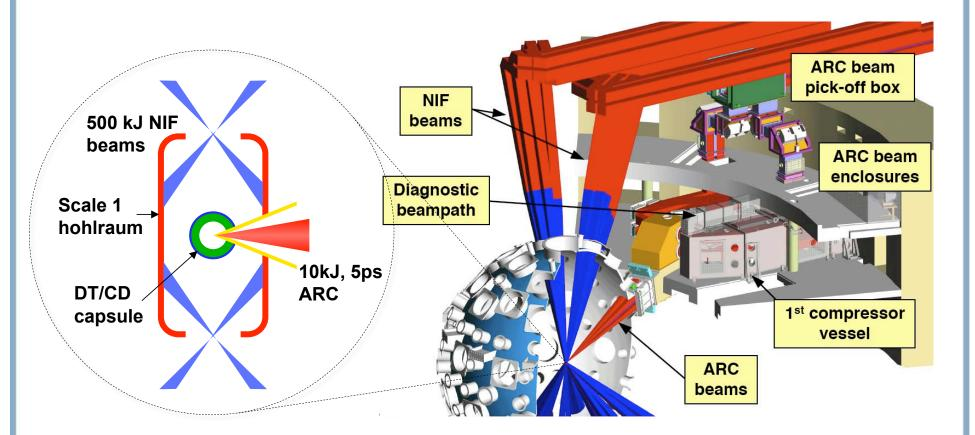
We will measure & optimise *coupling efficiency* of an 10 kJ ignitor pulse to a full-scale fuel assembly
