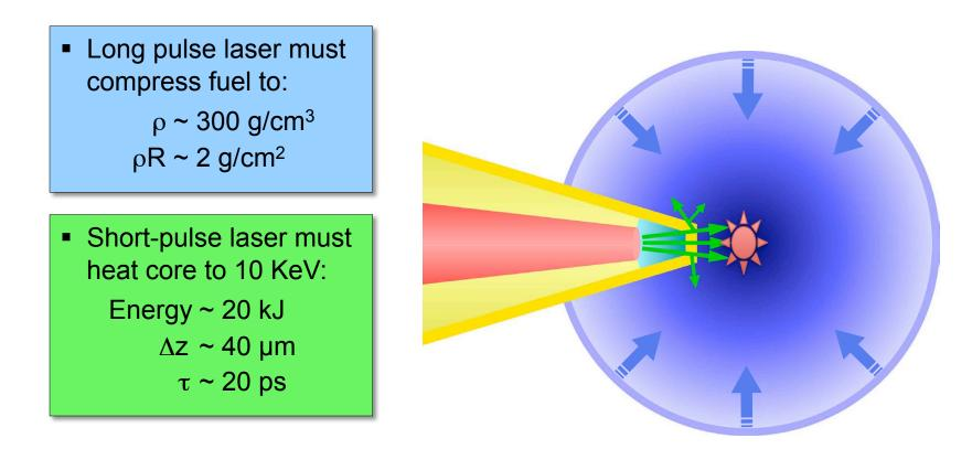
High-intensity, short-pulse lasers (I > 10<sup>19</sup> W/cm<sup>2</sup>) incident on a solid target can very efficiently accelerate intense beams of energetic electrons
