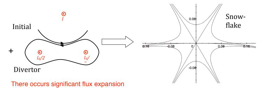
In addition to an exact snowflake, there exists a broad variety of "near-snowflake" configurations
