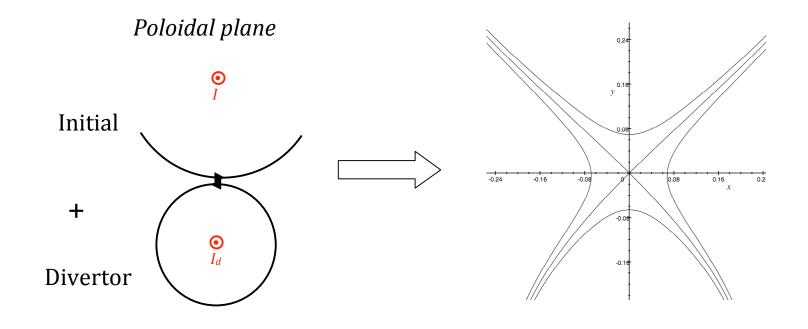
If one wants to make a second-order null of the poloidal magnetic field at a chosen point, one should design the divertor coils in such a way as to satisfy two conditions:
