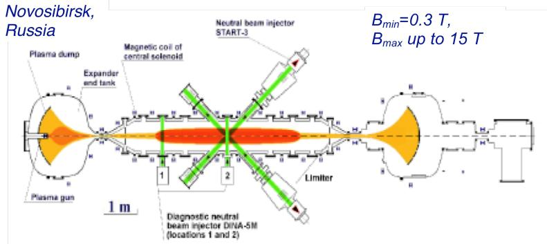
Fully axisymmetric plasma, MHD stable for beta 0.6 (60%), average ion energy 10 keV, average ion density 5×10<sup>13</sup> cm<sup>-3</sup>, no signs of the ion microinstabilities, electron temperature 200 eV, classical energy and particle confinement.
