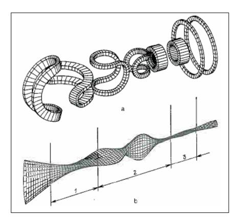
Stability by the set of quadrupole coils (MFTF-B, Livermore, 1980s)
