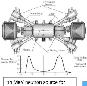
14 MeV neutron source for material and subcomponent testing
