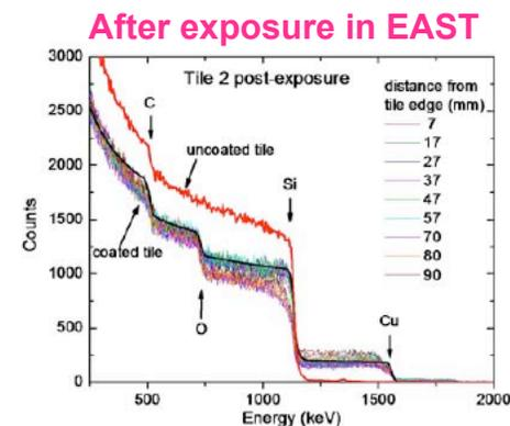
*Rutherford backscattering analysis of a tile with a 1 $\mu$ m C layer following erosion by >10hr plasma exposure in EAST tokamak (W. Wampler, 2011)*
