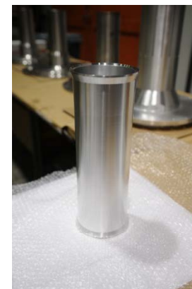
Actual deformable Aluminum liner for the next shot. (Slotted current return assemblies in the background)
