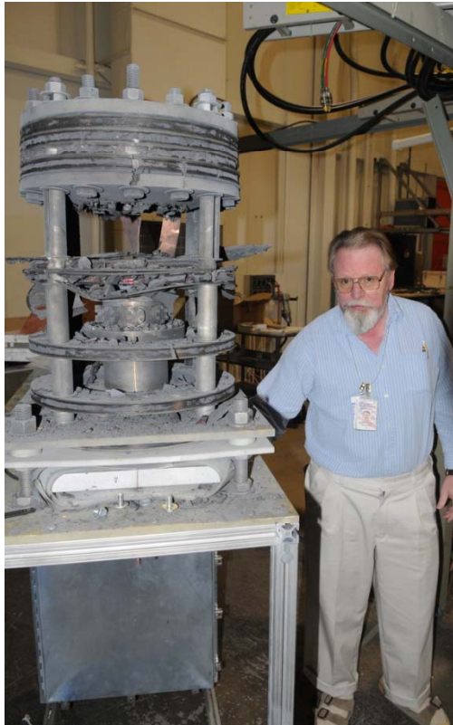
Project leader Jim Degnan next to remains of the coils from the second engineering test shot.
