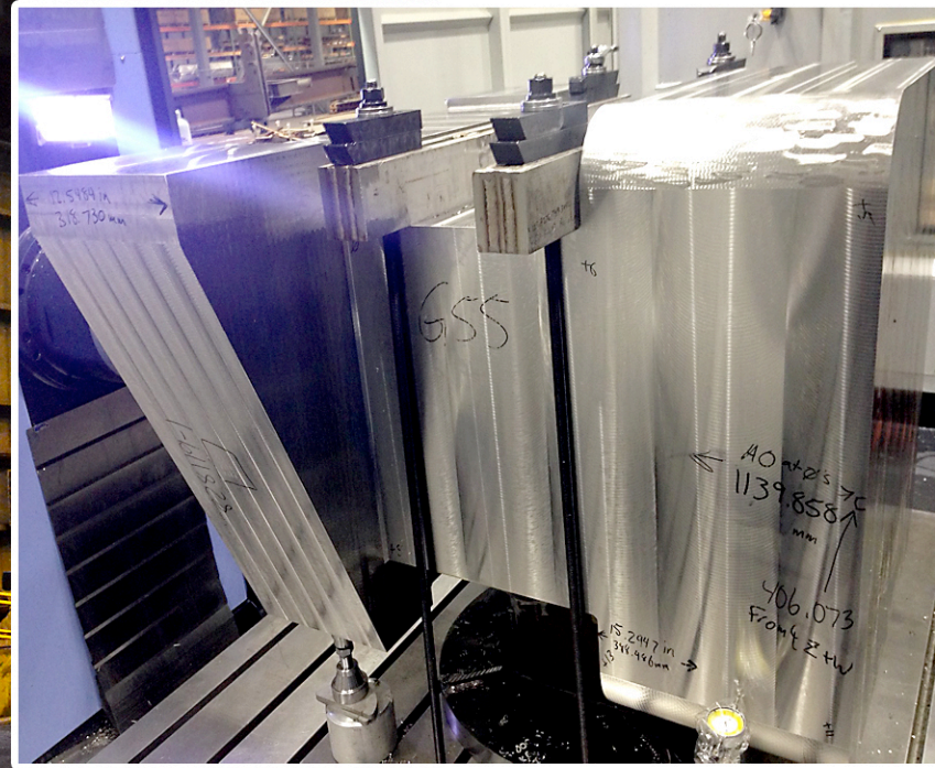
Lower key block during set-up for finish machining at Peterson, Inc. in Ogden, Utah.
