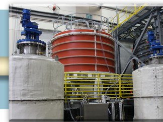
8: Vacuum Pressure Impregnation
