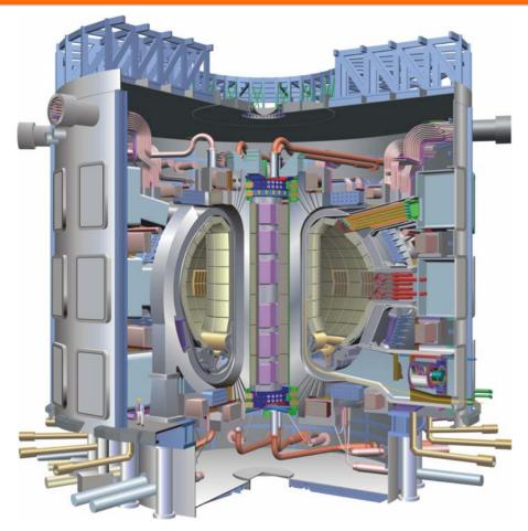
500 – 700 MW thermal fusion power 400 sec – 1 hr pulse length
