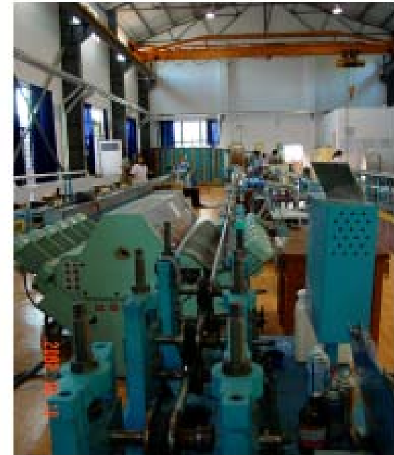
The jacketing line of Cable In Conduit Conductor (CICC)
