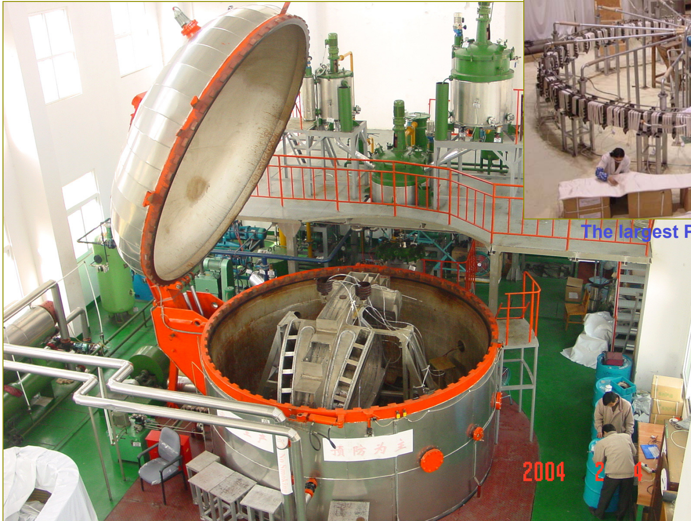
Vacuum impregnation workshop(VPI) for TF and PF coils
