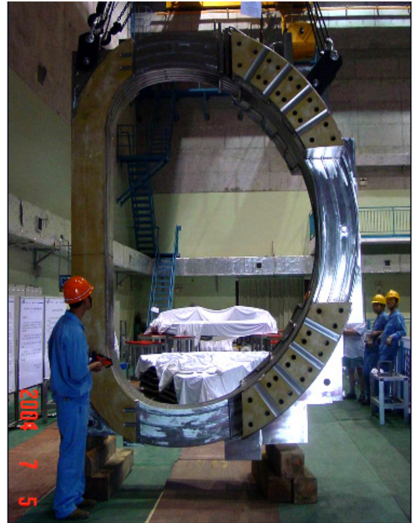
The TF magnets were ready for the final assembly
