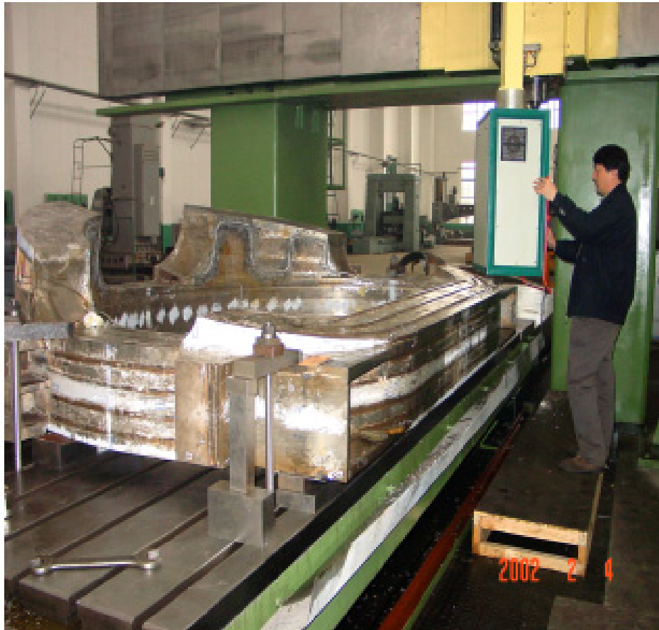
TF coil case is under machining by NC-milling machine
