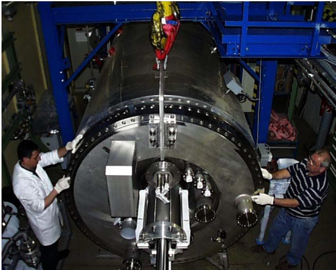
Figure 5.7-1 50% Scale Cryogenic Pump (EU)
