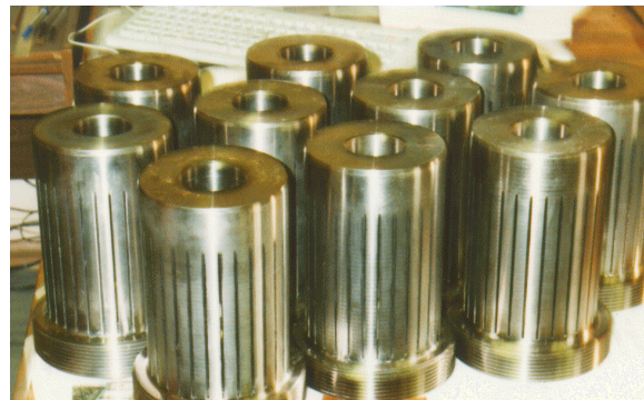
Figure 5.4-1 Flexible Mechanical Attachments made of Ti-Alloy (RF)
