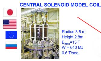
Radius 3.5 m Height 2.8m B<sub>max</sub>=13 T W = 640 MJ0.6 T/sec
