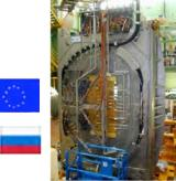
Height 4 m Width 3 m B<sub>max</sub>=7.8 T I<sub>max</sub> = 80kA
