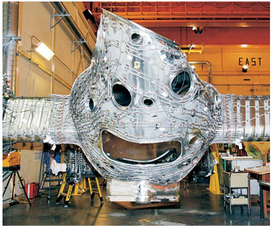
**The vacuum vessel** (segment shown) and other parts of the canceled stellarator at the Princeton Plasma Physics Laboratory have strange shapes to create quasi-symmetry for the plasma particles.
