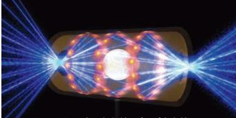
**Hot spot.** Beams heat the inside surface of the hohlraum, generating x-rays to explode the central fuel capsule.
