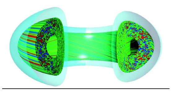
Figure 3.2. Contours of constant potential from a computer simulation of plasma turbulence in the DIII-D tokamak using the GYRO code. Note how the turbulent eddies are elongated along the magnetic field, while shear in the plasma  $E \times B$  rotation prevents structures with a cross-field dimensions greater than  $\sim 10^{-1}$  from forming. Courtesy of General Atomics.
