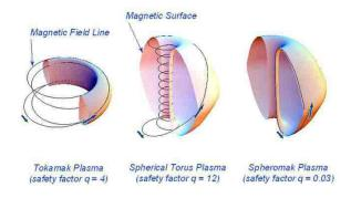
Figure F.2 Examples of the magnetic topologies of several related toroidal configurations with increasing curvature and varying stability characteristics. The tokamak (left) uses a strong external toroidal field to provide robust stability against pressure- and current-driven instabilities. The spherical torus uses a weak toroidal field in a compact configuration to allow access to higher  $\beta$  values than obtained in the tokamak.
