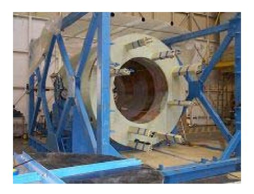
Figure 3.7 ITER Central Solenoid Model Coil that achieved 13 T and x.x T/s ramp rate (1/2 scale of full coil). Courtesy of ITER.
