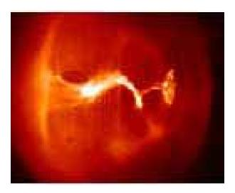
Figure 2.3 Kink instability of central column produced in Caltech spheromak formation experiment. This kink, believed intrinsic to spheromak self-organization, occurs when the jet-like central column becomes sufficiently long to satisfy the Q=1 Kruskal-Shafranov instability threshold. It can also be considered as a good simulation of the kink instability of an astrophysical jet. Courtesy of S. C. Hsu and P. M. Bellan, California Institute of Technology.
