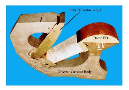
Figure 3.8 Prototype ITER Divertor Plasma Facing Component. Courtesy of ITER.
