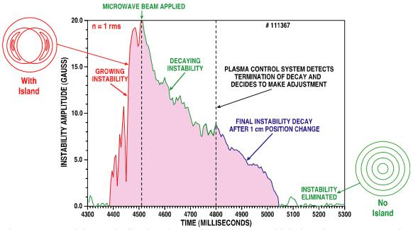
Figure 3.4 Applying and adjusting the precise position at which the microwave power is deposited stops the growth of a neoclassical tearing mode, and then eliminates it. Courtesy of General Atomics.
