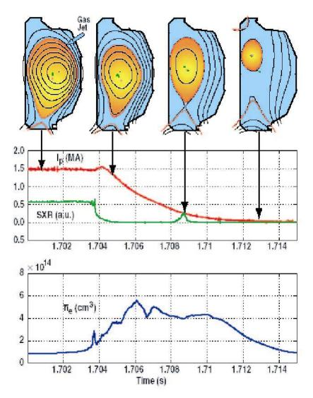
Figure 3.5. The controlled termination of a DIII-D discharge by injection of a nobel gas. This technique holds great promise as a means of mitigating damage which might otherwise occur during off-normal event in ITER. Courtesy of General Atomics.
