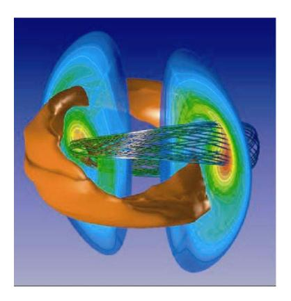
Figure 3.3 A spherical tokamak with a saturated magnetic island due to sheared toroidal rotation. Calculated by the M3D code. Courtesy of W. Park, Princeton Plasma Physics Laboratory.
