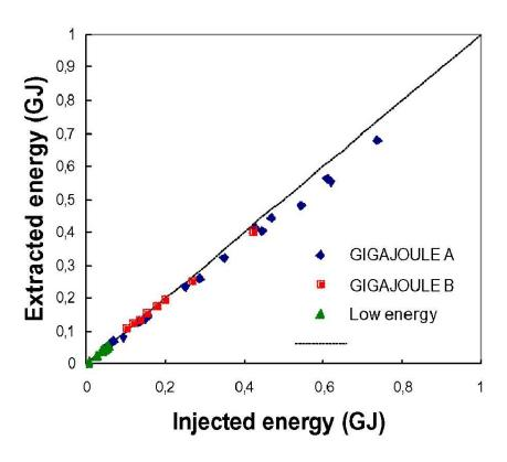
Figure 3.9 Results of experiments using an actively cooled limiter on Tore Supra. Courtesy of J. Jacquinot, Euratom-CEA Association, CEA Cadarache; Tore Supra, France; and IAEA. Ref. *Recent Developments Towards Steady State Physics and Technology of Tokamaks in Cadarache* J. Jacquinot. Proceedings of the 19th IAEA Fusion Energy Conference, Lyon, October 2002.
