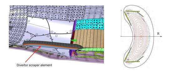
Figure 3: Divertor scraper elements will protect the throat (narrowest part) of the divertor against heat transients during evolution of the plasma beta. The magnetic configuration near the island divertor plates, is shown on the right.
