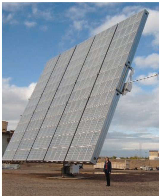
Scope of the problem. This concentrator photovoltaic collector can generate 138 kilowatt-hours per day, half the energy consumption of an average American.
