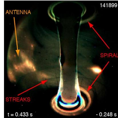
**Figure 2** - During RF heating on NSTX, bright streaks can emerge from the antennas and terminate in bright and hot spirals in the upper and lower divertor regions, indicating that a significant fraction of the RF power couples directly to the SOL and is subsequently lost to the divertor regions.
