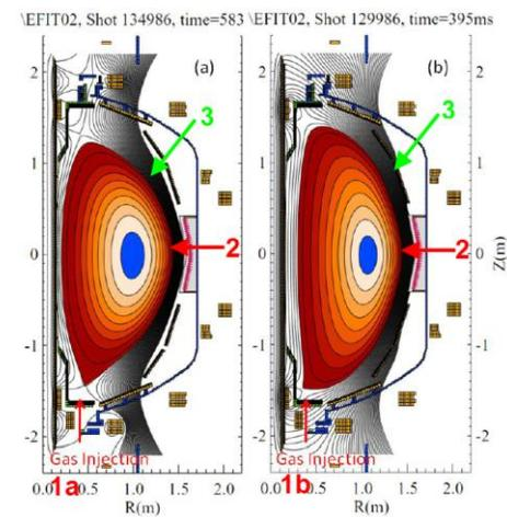
Figure 6 - Planned Massive Gas Injection locations on NSTX-U. (1a) Private flux region, (2) mid-plane injection, (1b) high field lower SOL region and (3) outer SOL above the mid-plane.
