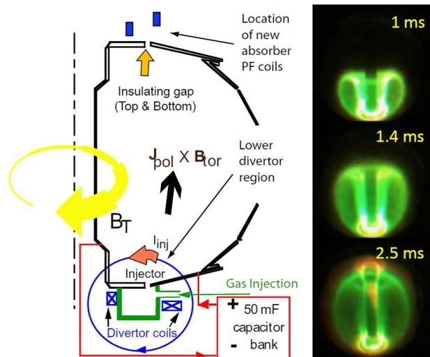
Figure 13 – (left) schematic and (right) camera images of Coaxial Helicity Injection (CHI) plasma start-up in NSTX.
