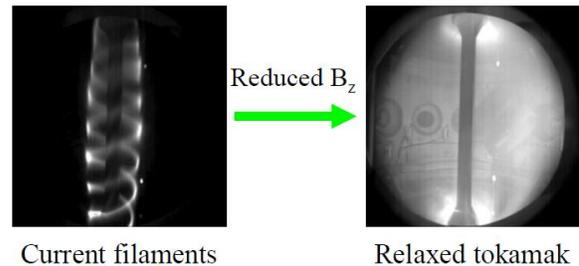
Figure 14 – Example of point helicity injection plasma current start-up on the Pegasus Toroidal Experiment.
