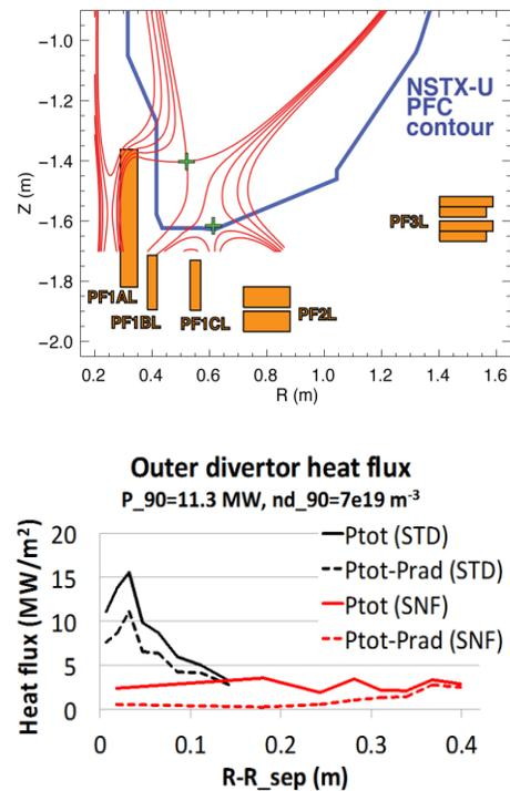
Figure 11 - Snowflake divertor geometry in NSTX-U (top panel), divertor heat flux profiles in standard (STD) and snowflake (SNF) divertors (bottom panel)
