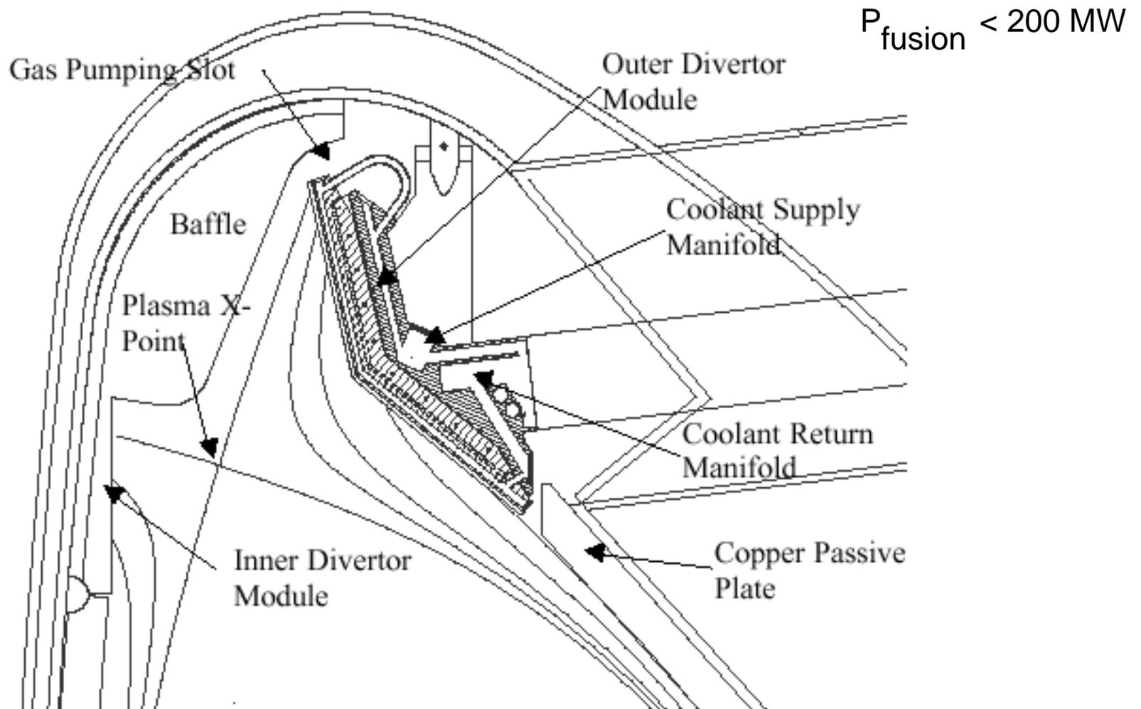
Reference Design is semi-detached operation with  $<15 \text{ MW / m}^2$ .
