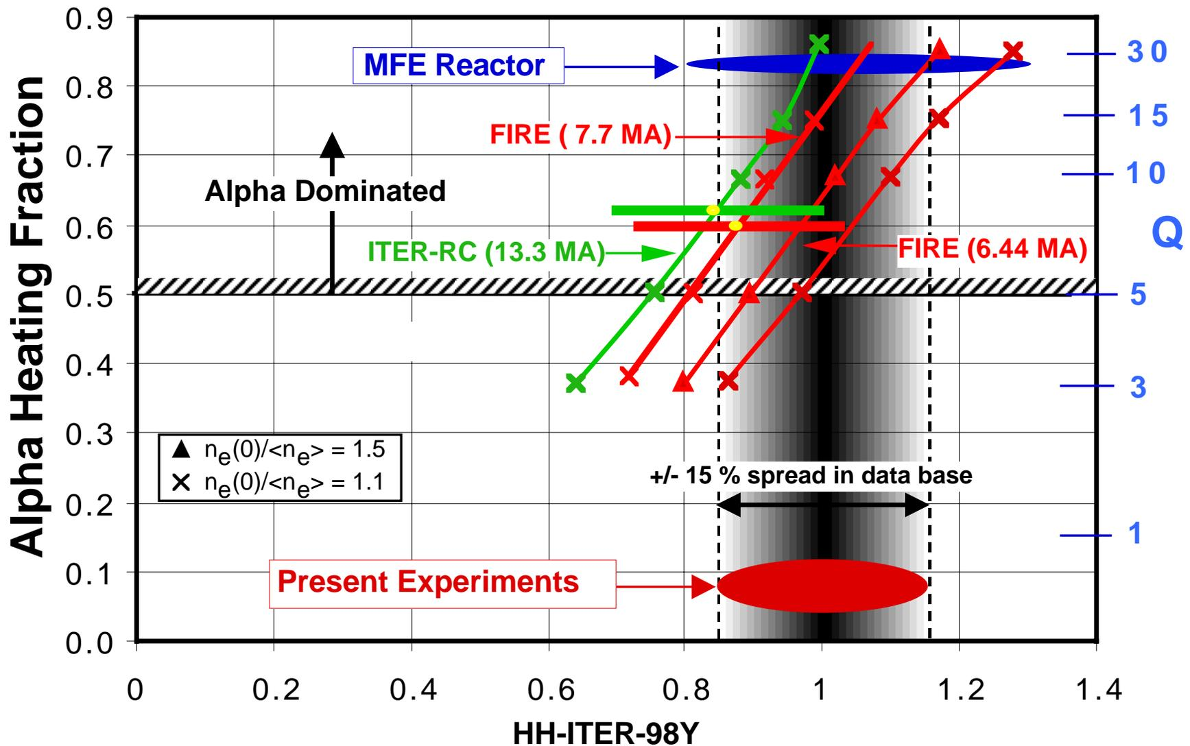
The dynamics of a burning plasma is determined by the alpha heating fraction which is not subject to a sharp threshold versus confinement.
