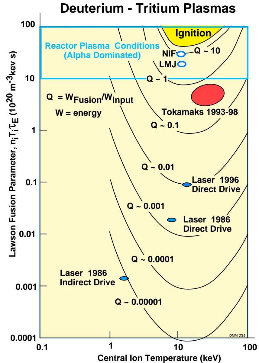
Only the tokamak is sufficiently advanced to permit the design, construction and initiation of a next step burning plasma experiment within the next decade that could address the alpha-dominated burning-plasma physics issues of magnetic fusion.
