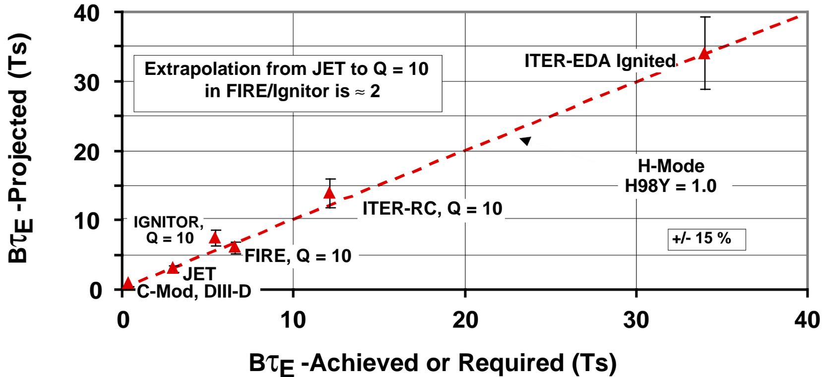
High magnetic field allows FIRE and IGNITOR to operate at high density, thereby reducing the required extrapolation in confinement, the most uncertain quantity.
