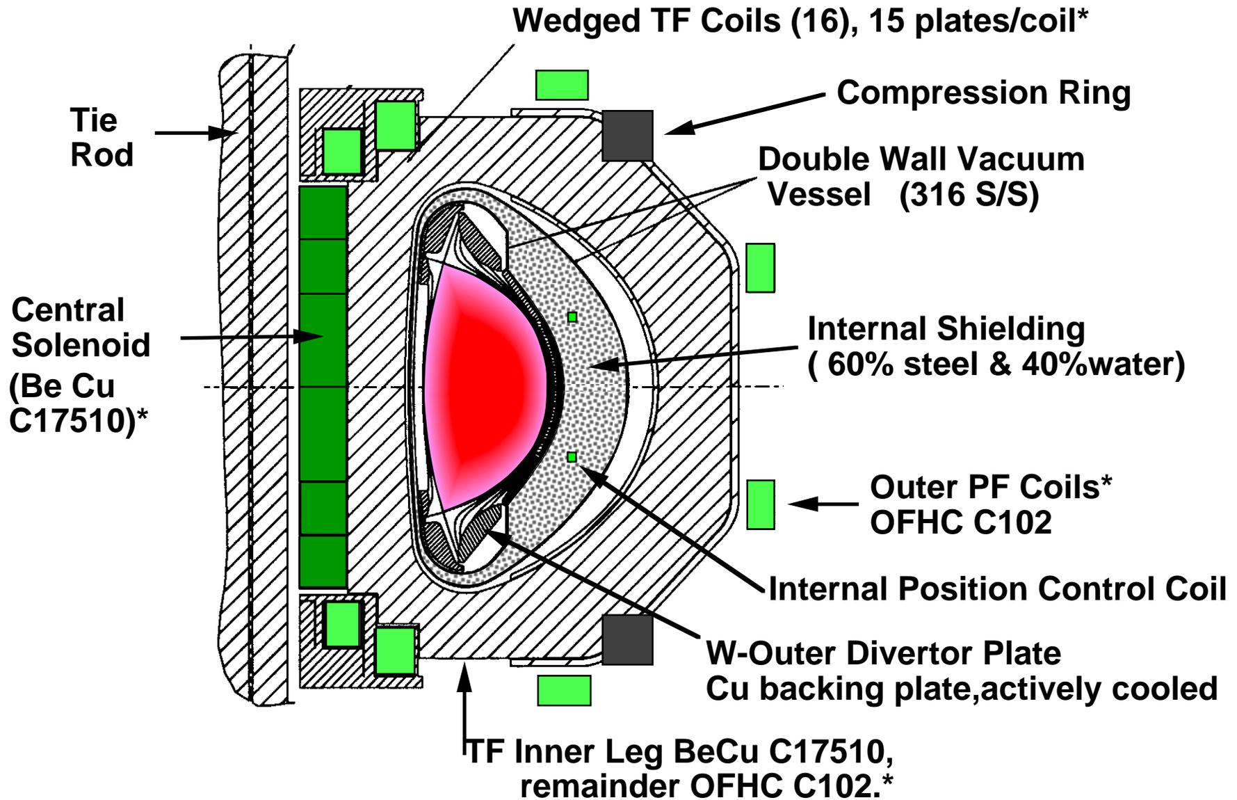
\*Coil systems cooled to 77 °K prior to pulse, rising to 373 °K by end of pulse.
