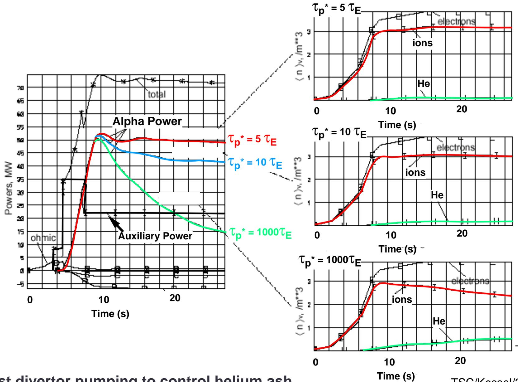
Adjust divertor pumping to control helium ash
