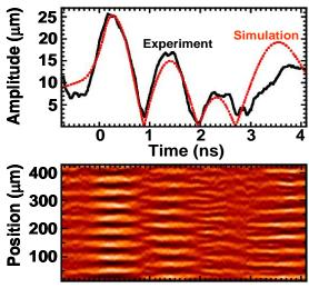
Precise understanding of hydro-instability is important for both indirect and drive ignition designs.
