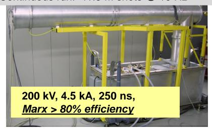
Mechanisms that limited lifetime of Electra's plasma-cathode diode were identified and corrected on Electra (up to 100,000 shots.) All solid state pulse power would allow much longer run times & tests.
