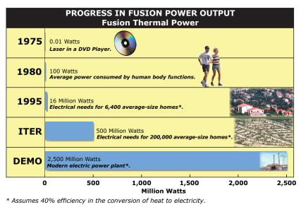
physics experiments, which produced up to 16 million watts of fusion heat for time periods approaching one second, to a Demonstration Power Plant (Demo) producing 2,500 million watts of fusion heat (1000 million watts of electricity) continuously with a gain of over 25.
