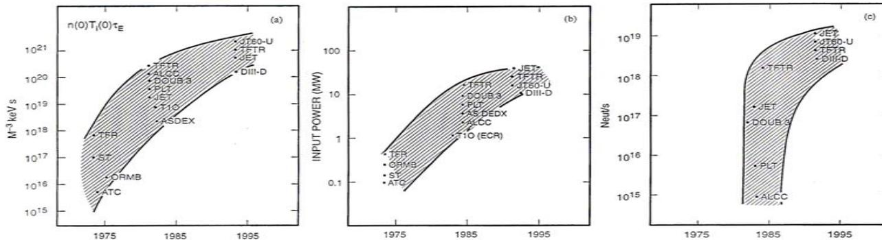
Figures of merit for recent tokamaks: (a) triple fusion product, (b) input power, and (c) D-T neutron production rate.
