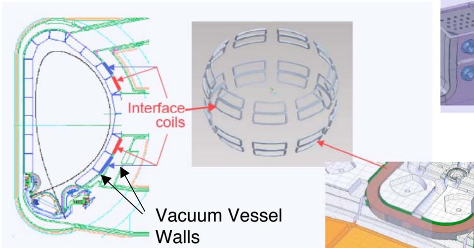
**(4 rows x 9 toroidal) Blanket-Vessel Interface Coils**
