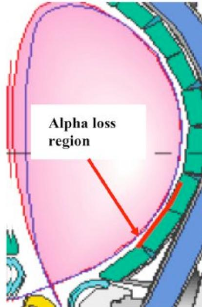
First wall region marked by the thick red line undergoes  $\alpha$  particle bombardment due to TF ripple loss
