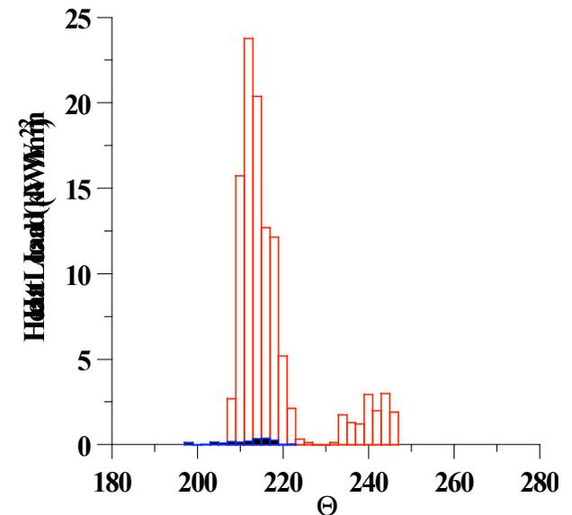
Poloidal distribution of heat load due to banana particle loss (red) and locally trapped  $\alpha$  loss (blue)
