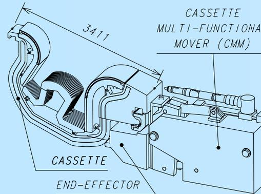
**Multifunction manipulators are used for divertor cassette removal and to handle vacuum vessel port plugs. A toroidal mover slides the divertor cassettes along rails into their final position.**
