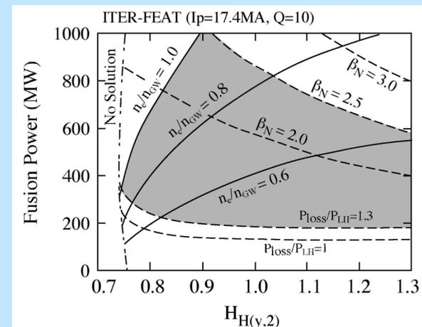
The combination of a range of plasma parameters will allow  $Q=10$  to be obtained. The figures show the operational domain in terms of fusion power and  $H_H$ , plus the various limiting boundaries that are thought to apply.
