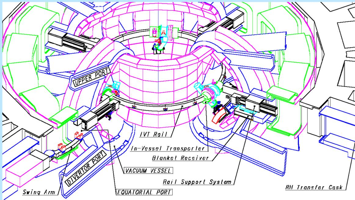
Systems near the plasma will become radioactive and will require remote maintenance, with special remote handling equipment. In-vessel transporters are used to remove and reinstall blanket modules.
