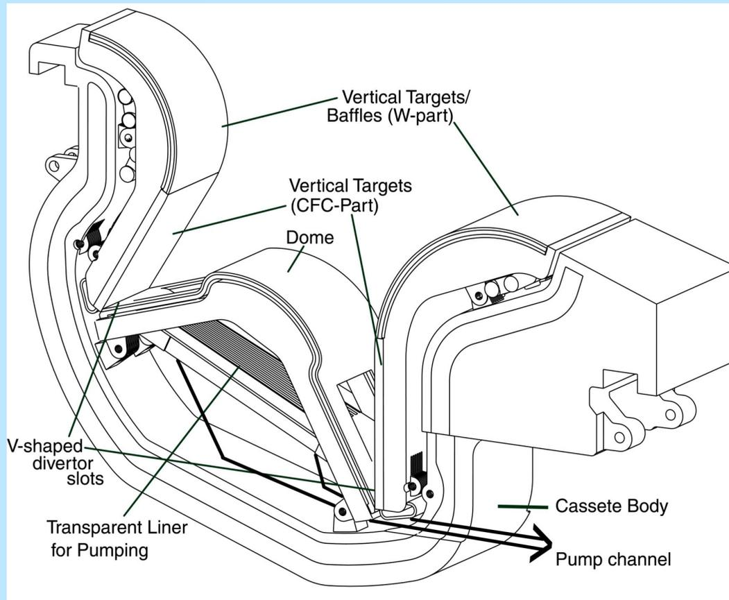
The divertor is made up of 54 cassettes. The target and divertor floor form a V which traps neutral particles protecting the target plates, without adversely affecting helium removal. The large opening between the inner and outer divertor balances heat loads in the inboard and outboard channels.
