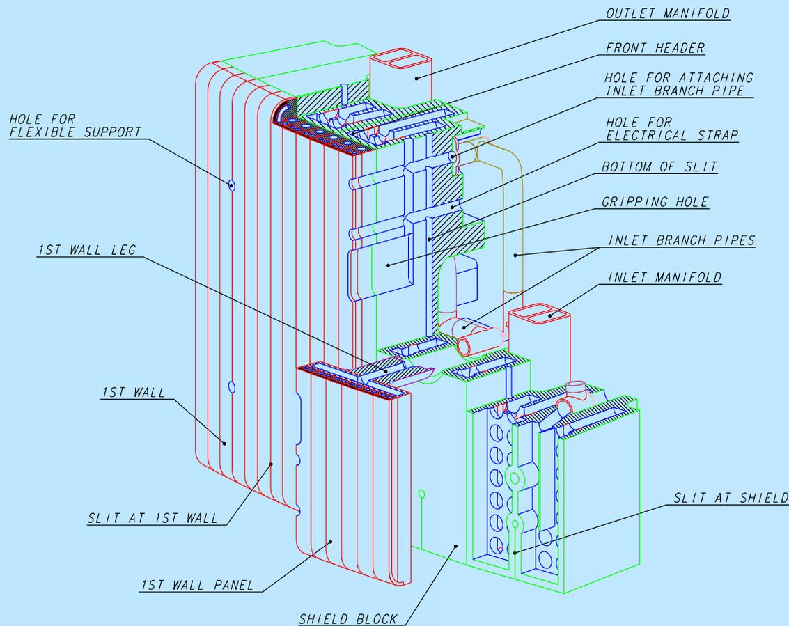
The ~ 420 blanket modules consist of a detachable faceted first wall (FW) built with Be armour and a water-cooled copper heat sink attached to a SS shielding block. This minimises radioactive waste and simplifies manufacture. The blanket cooling channels are mounted on the vessel.
