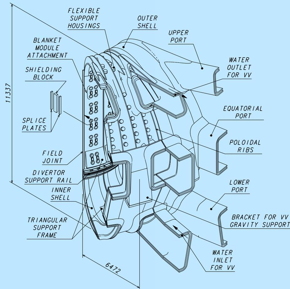
The primary functions of the vacuum vessel (VV) are to provide a high quality vacuum for the plasma, as well as the first confinement barrier to radioactive materials and a second barrier (after the cryostat) for the separation of air from potential sources of in-vessel hydrogen generation.
