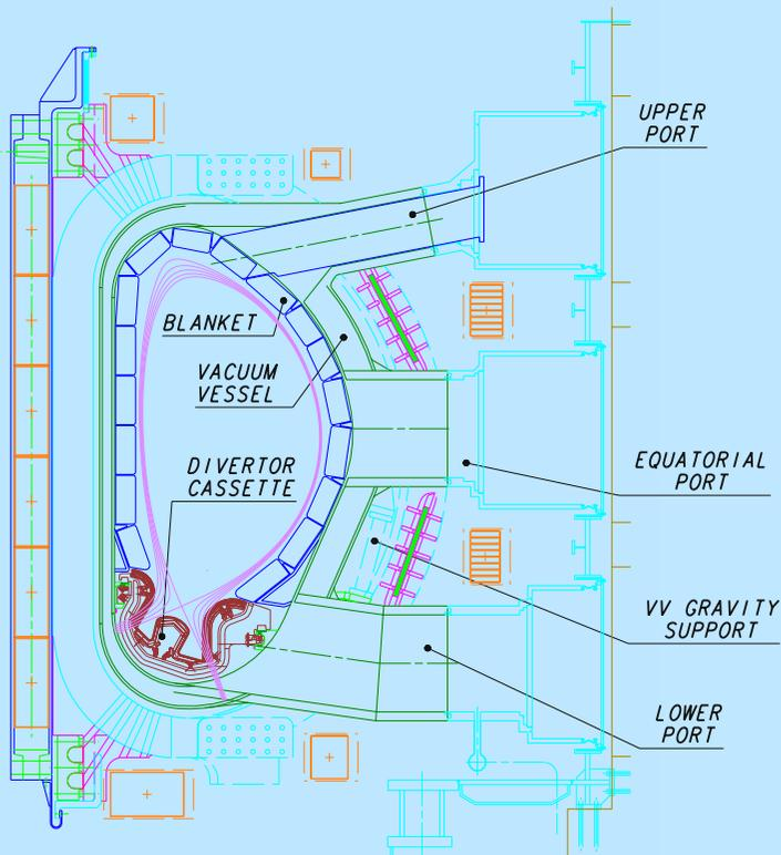
The double-walled vacuum vessel is lined by modular removable components, including blanket modules, divertor cassettes, and diagnostics sensors, as well as port plugs for limiters, heating antennae, diagnostics and test blanket modules. All these removable components are mechanically attached to the VV. The total vessel/in-vessel mass is  $\sim 10,000$  t.
