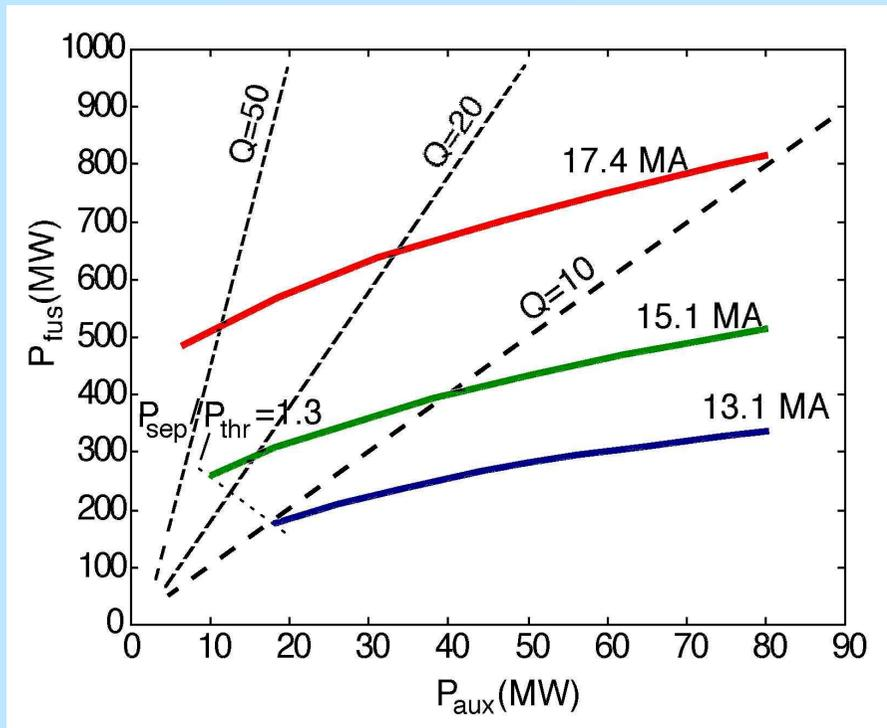
Fusion power ( $P_{fus}$ ) versus auxiliary power ( $P_{aux}$ ) for a range of currents and for  $H_H = 1$  and  $n_e/n_{Greenwald} = 0.85$ . Minimum fusion power is limited to a factor 1.3 above the expected power at which transition to L-mode would occur, namely:
