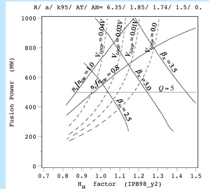
Operation space for  $I_p = 12$  MA and  $P_{CD} = 100$  MW, in terms of fusion power versus confinement enhancement factor, and the transition from hybrid to true steady-state operation.
