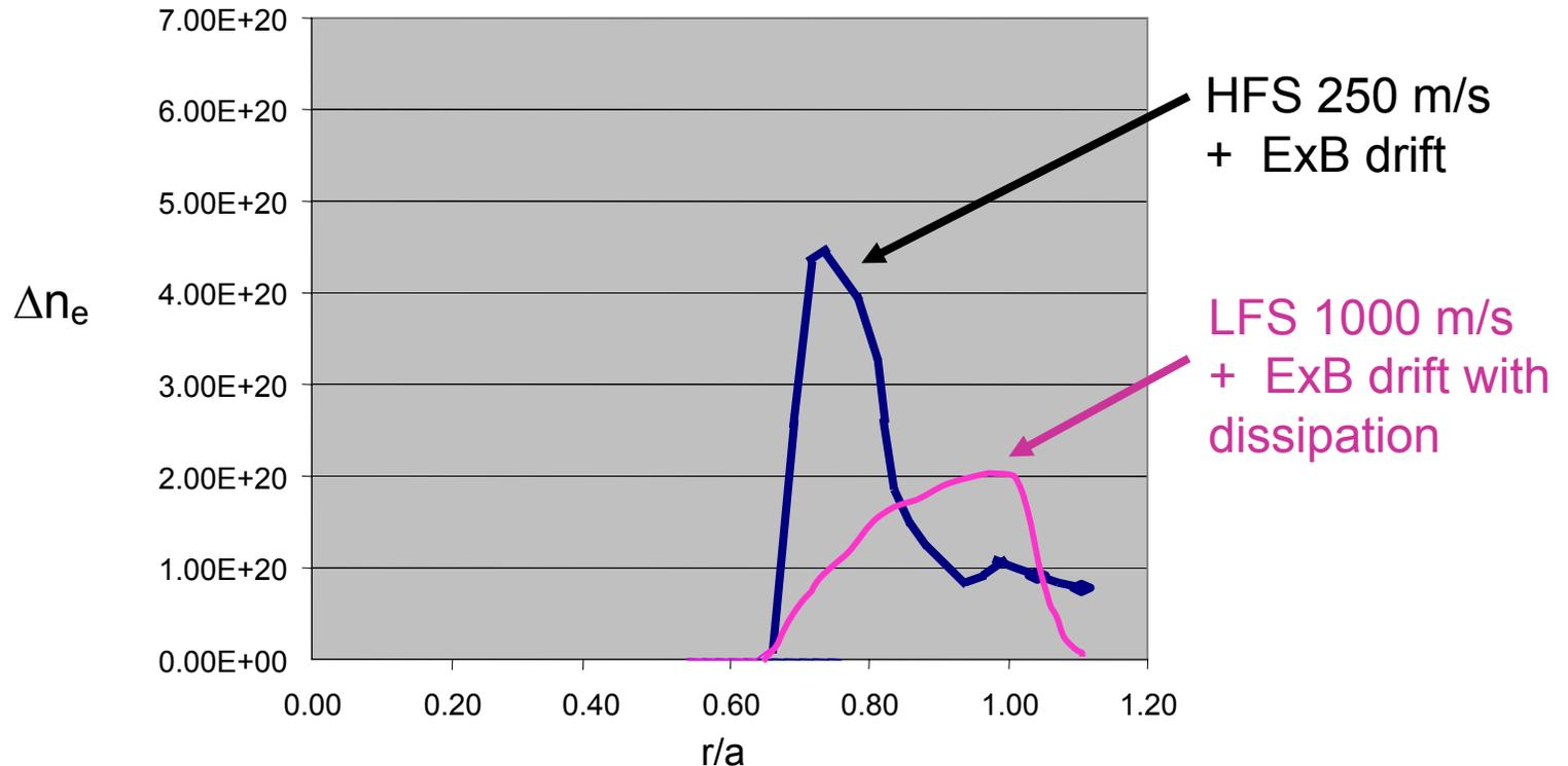
The resulting deposition from a 4 mm pellet injected from the outside midplane (LFS) and inner wall (HFS) including ExB drift effects to NGS pellet ablation. The calculation uses the Pellet Relaxation Lagrangian code to model the cloudlet displacement from ExB drift. Dissipation is ad hoc scaled from DIII-D results.
