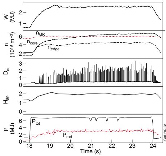
Fig. 2. The time evolution of a typical pulse 48276; the traces are (1) the stored energy (2) the core line average density, the edge line average density ( $R = 3.78$ ) and the Greenwald density (3) the  $D^\alpha$  emission (4) the  $H_{89}$  ratio ( $\equiv \tau_E/\eta_{TER89}$ ) (5) the total power input and the radiated power.
